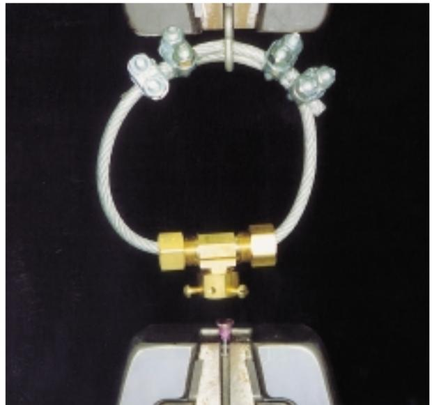
**Fig. 5** Test jig with 3 side screws attached to the universal testing machine to test the cement failure load.
