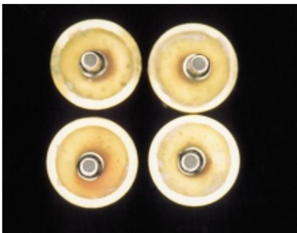
**Fig. 3** Acrylic resin used to fix the abutment/analog assembly in the mounting jig.
